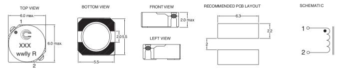
Dimensions are in millimeters.
